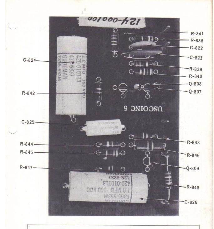
VIBRATO RECOVERY AMPLIFIER BOARD SERIAL NO. 15000 AND UP SCHEMATIC FIGURE 49 FIGURE 38
